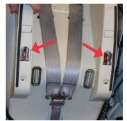
On bottom of carrier where rubber strips run along edges of support rails, there is an exposed opening with attachment hooks.
